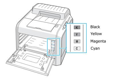
**20** Holding each toner cartridge, insert them into their corresponding positions shown in order of Cyan, Magenta, Yellow and then Black. Using both hands, grip the cartridge to insert into the slot. Then hold the handle to slide the cartridge in.
